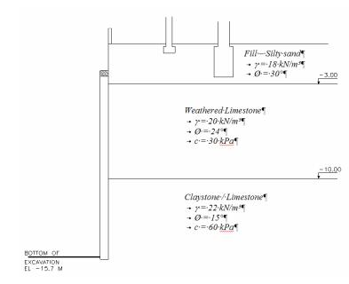
Fig. 2. Typical soil profile and design characteristics
