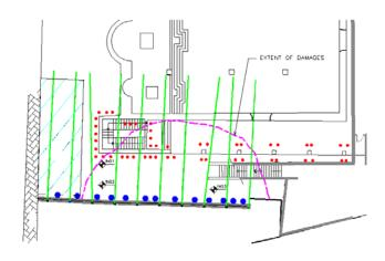
Fig. 3. Extent of 'failed zone" and micropile layout
