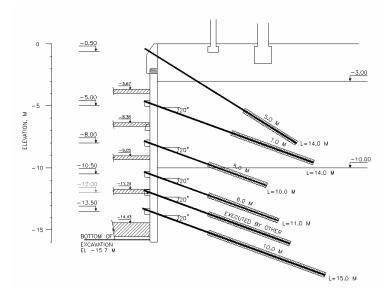
Fig. 6. Layout of the re-designed shoring system along lot-235
