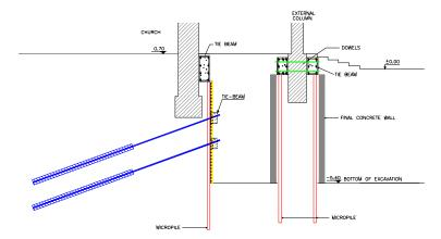
Fig. 5. Shoring and underpinning for the multi-purpose hall
