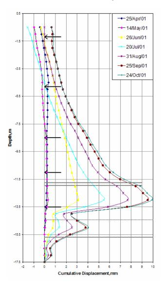
Fig. 7. Cumulative displacements at IN02
