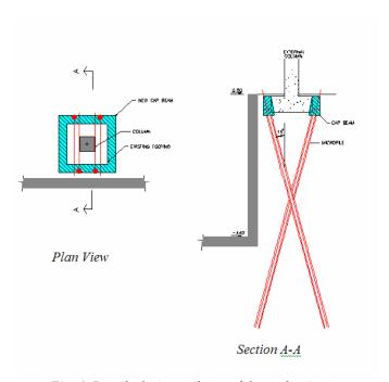
Fig. 4. Detail of micro-piles used for underpinning
